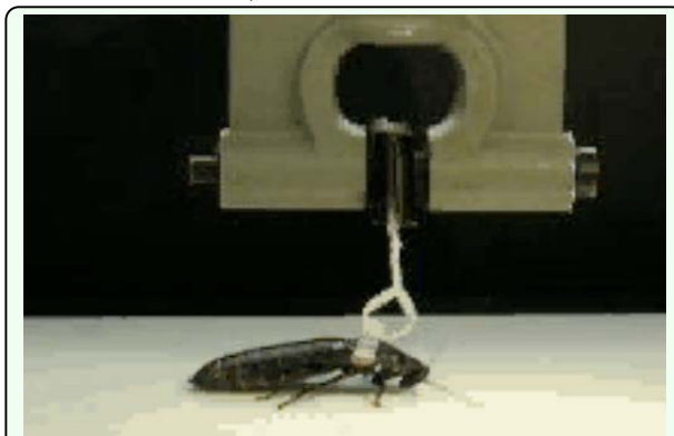
Video of experimental protocol during adhesion testing of Gromphadorhina portentosa using the Instron® universal testing machine. Filename: vancasteren_codd_experimental_testing The video file is available online.
