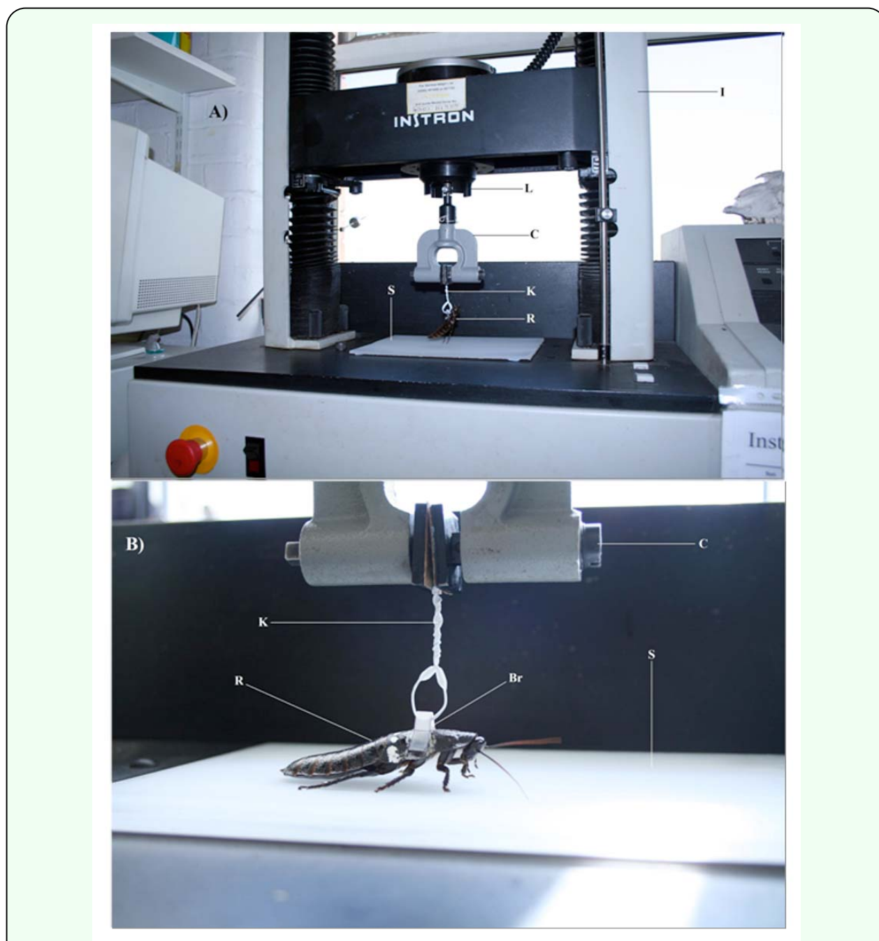
Figure 1. Experimental setup for peak force experiments. A) Instron universal testing machine, B) Close-up of attachment of Gromphadorhina portentosa to the load cell. Labels: C = Clamp, S = Sample substrate, Br = Bracket, K= Kitchen twist tie, R= G. portentosa , L = Load cell, I = Instron® machine. Pictures taken by AvC. High quality figures are available online.
