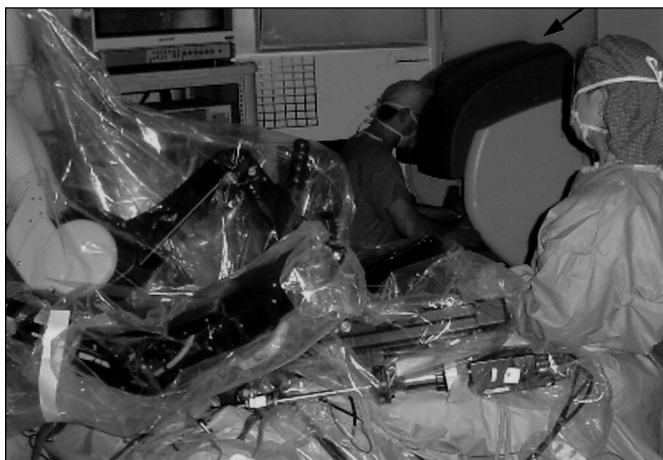
Figure 2. Intraoperative photograph of the da Vinci system with surgeon's console (arrow), vision cart (double arrow) shown in the background, and surgical cart with robotic arms visible in the foreground.
