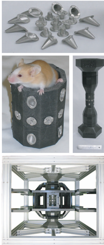
Fig. 4. FastSPECT III imaging aperture fabricated using 3D rapid-prototyping printers and casting techniques. Top: platinum pinhole inserts made by lost-wax casting methods; Middle: (left) cold-cast tungsten composite aperture with pinhole inserts, (right) complete imaging aperture; Bottom: imaging aperture installed in FastSPECT III frame.
