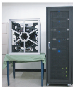
Fig. 6. Complete FastSPECT III imaging system with acquisition/processing computers. CCD data from all cameras are acquired and processed simultaneously.
