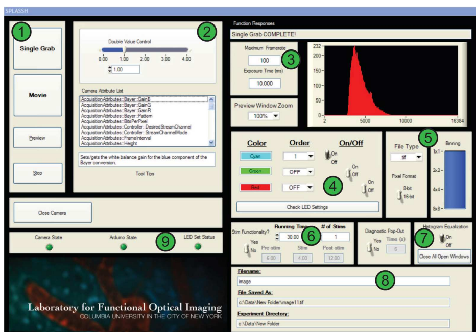
Fig. 2. The SPLASSH Graphical User Interface provides a single window from which to control all aspects of multispectral and fluorescence imaging acquisition. The GUI is organized into panels which contain buttons that access similar types of high-level routines (see Section 3.2 for descriptions). Acquired images are displayed in their own pop-up windows, separate from the control GUI. When initializing the program, SPLASSH dynamically communicates with the camera to determine its capabilities and available camera properties. SPLASSH then updates the corresponding GUI interfaces to reflect these values (e.g. the number of available binning modes).
