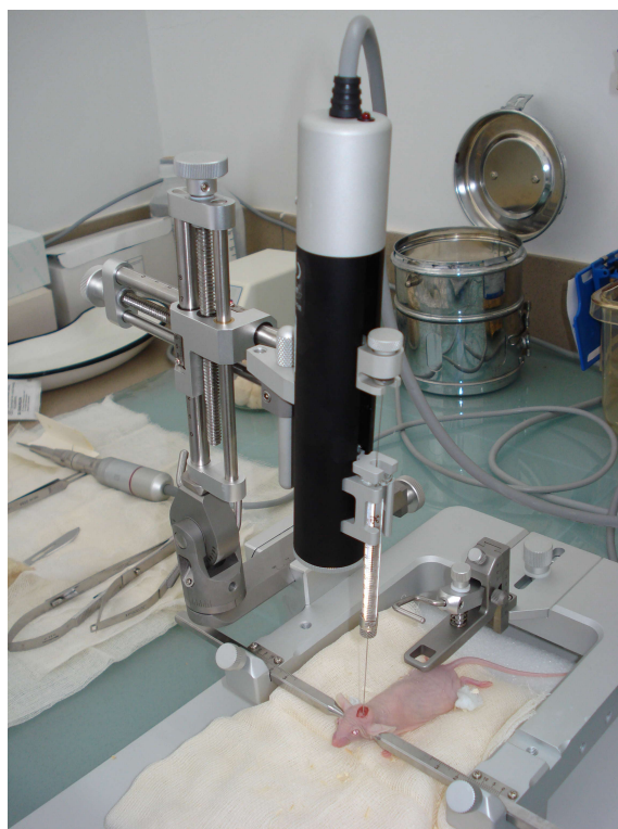
Fig 6: Stereotaxic system: TAXIC-600 - WPI Stereotaxic Frame 18 deg. Ear Bars and UMP 3-1 injection system, (World Precision Instruments, Germany).
