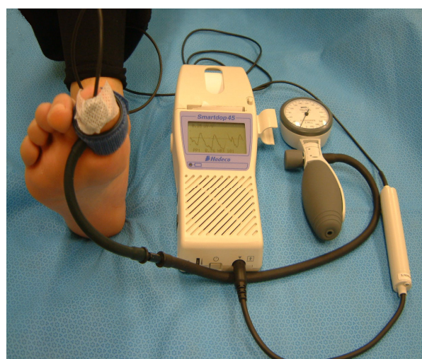
Figure 1 Measurement of Toe Systolic Pressure using a manual PPG unit (Hadeco Smartdop 45)™.
