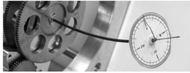
Fig. 12. Tube pair showing graduated disk, twist pointer, and tangent pointer.
