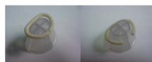
Fig. 8. SMP annuloplasty ring shown in its (left) primary and (right) temporary forms. The ring is shown on the base used to set the temporary shape. (Reprinted with permission from A. D. Lantada, P. LaFont, I. Rada, A. Jimenez, J. L. Hernandez, H. Lorenzo-Yustos, and J. Munoz-Garcia, Active Annuloplasty System for Mitral Valve Insufficiency, in BIOSTEC 2008, CCIS 25 , ed. A. Fred, J. Filipe and H. Gamboa, Springer-Verlag, Berlin, 2008, pp. 59–72.91)
