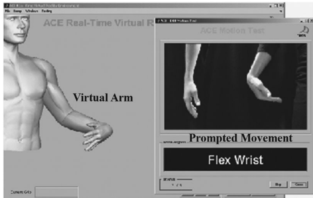
Fig. 2. The graphical user interface used for real-time testing. The prompted movement is shown on the right and the virtual arm is shown on the left.
