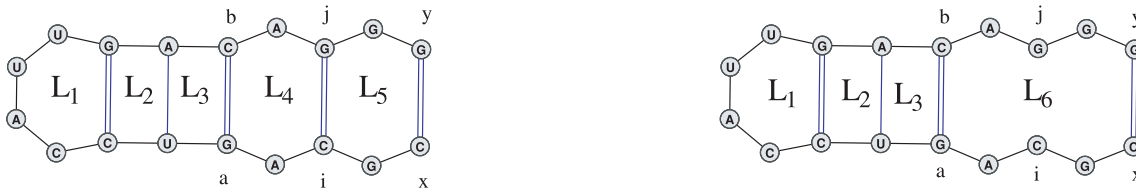
Figure 10. Example structure in recursion. The energy change effected by removing the base pair (i,j) is E(L_6) - (E(L_5) + E(L_4)) . To calculate this, we need to keep track of base pair (a,b) . Images created using the software VARNA [50]. doi:10.1371/journal.pone.0016178.g010
