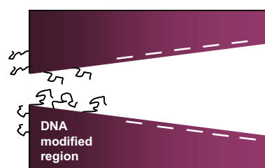
Fig. 1 Scheme of the surface charge pattern obtained in the process of one-sided modification of a single conically shaped nanopore with point-tethered DNA molecules. We estimate the position of the junction between the DNA-modified zone and the zone with carboxyl groups to be several tens of nanometers from the small opening of the pore (Vlassiuk and Siwy 2007). Carboxyl groups are formed in the process of pore preparation
