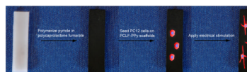
Figure 1. Schematic overview of the project's main steps: fabrication of PCLF-PPy composite scaffolds, cell seeding, and application of ES treatment regimens.
