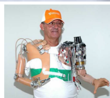
Fig. 1. On left side: (A) Three-DOF prosthesis consisting of nonpowered locking shoulder, passive humeral rotator, powered elbow, powered wrist rotator, and powered hook terminal device;
