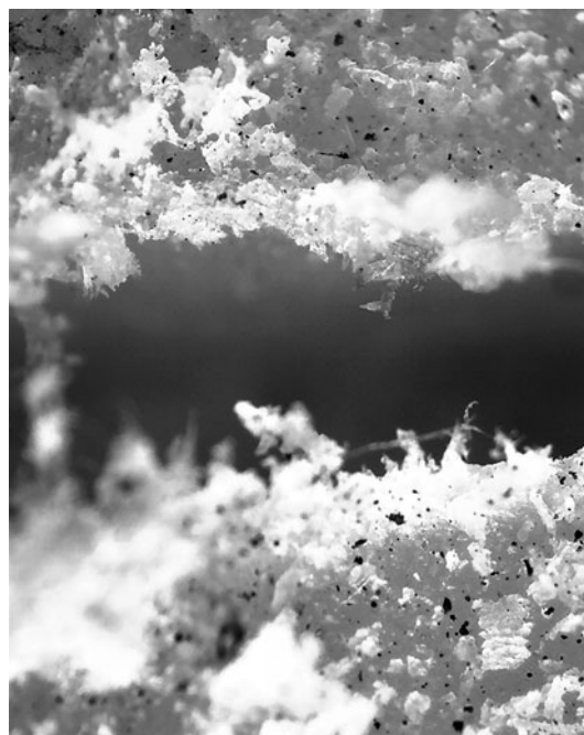
Fig. 14 Hand saw blade kerf
