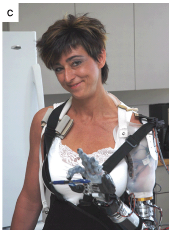
Figure 7. Patients using experimental arm prostheses. (a) Patient S2 was shown reaching to catch a tissue box using the DEKA arm. (b) Patient S1 was shown moving a ring across a geometric wire using the JHUAPL arm. (c) Patient T5 was shown grabbing a pen using the DEKA arm.
