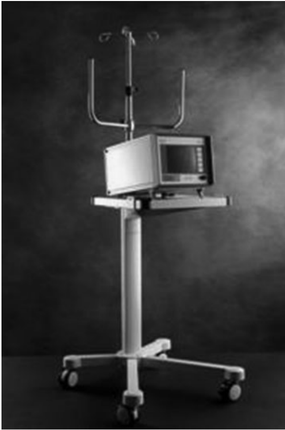
Figure 2 The EKOS Control Unit adjusts power input to the ultrasound transducers.
