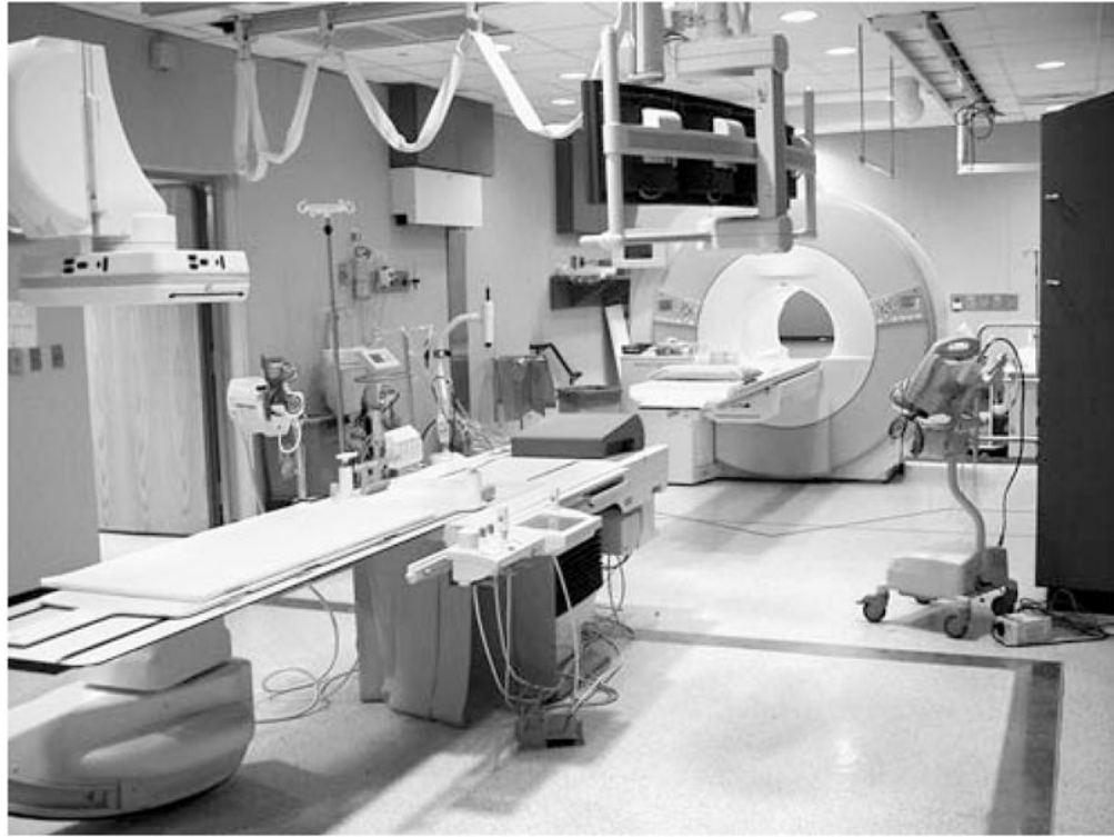
Fig. 6. Digital image of a combined X-ray angiographic and MR imaging suite with a flat-panel angiographic display and 1.5T clinical MRI scanner (Siemens Medical Systems). The table top can be transferred between MRI and X-ray to allow registration of the two imaging modalities. Such suites offer the advantages of high temporal resolution from X-ray fluoroscopy and high anatomical detail from MRI for cardiac interventions. Similarly configured suites are available from all major MRI vendors
