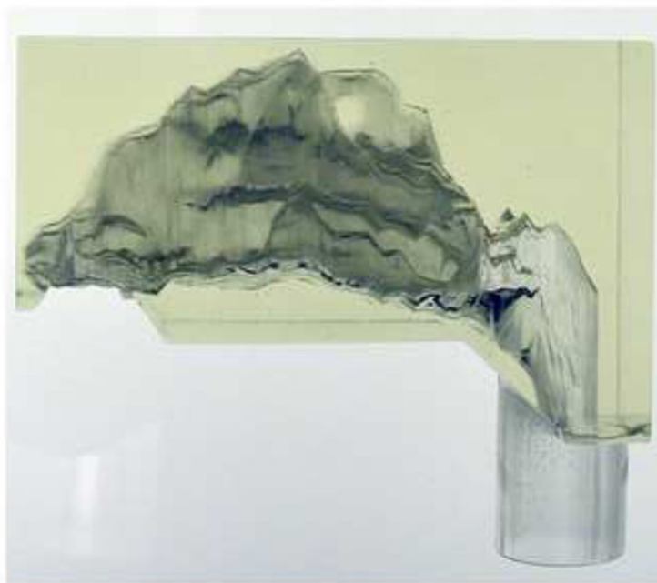
Figure 1. Photograph of the nasal replica used in the experimental particle deposition study of Kelly et al. (2004b).
