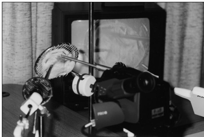
Figure 4. Lap-Ring Simulation Trainer with TS at 110° and television monitor in background.
