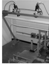
Fig. 2. The needle steering device inserts the needle into phantom tissue while the needle tip position is tracked using two overhead cameras.
