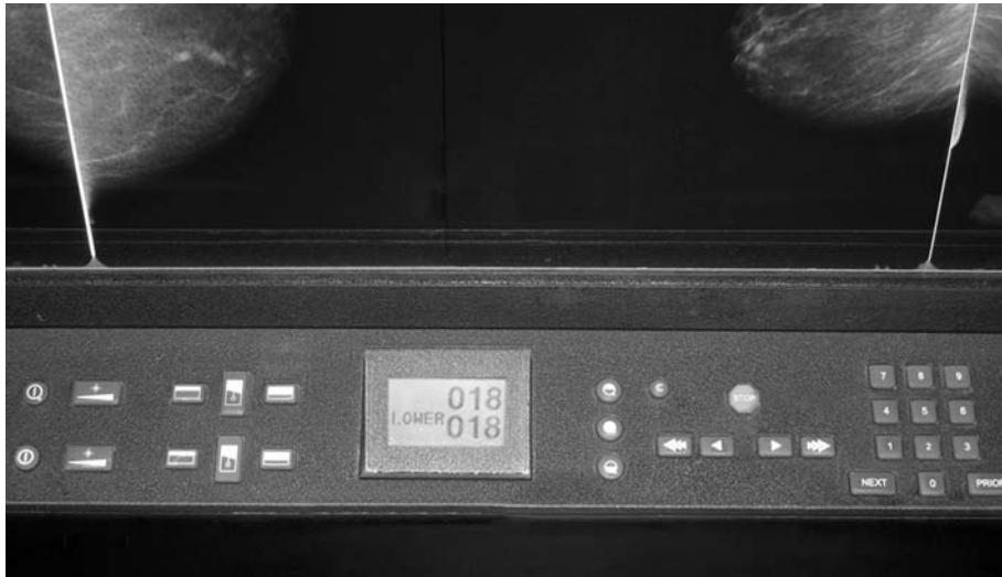
Fig 4. Photograph of the control panel of the alternator. All control buttons are clustered in the middle third of the table. The button marked next moves both the top and bottom film holders to the next panel and stops them there.
