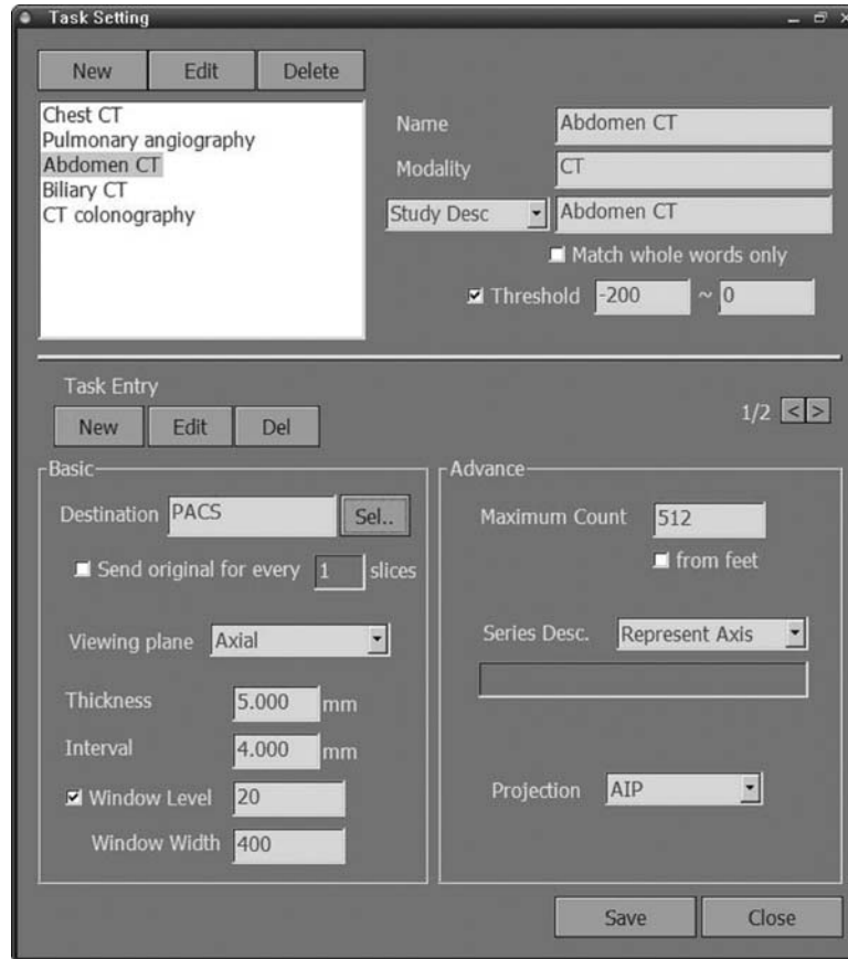
Fig 1. Configuration of the reformation parameters. For a study with the Study Description Abdomen CT , a set of axial MPR images is generated with a 5-mm slab thickness, a 4-mm interval, an average intensity projection, a window width of 400, and a window center of 20.
