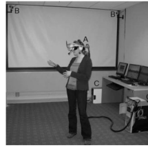
Figure 1. Illustration of immersive virtual environment equipment. A) Head-mounted display; B) Tracking Cameras; C) tracking and rendering computers
