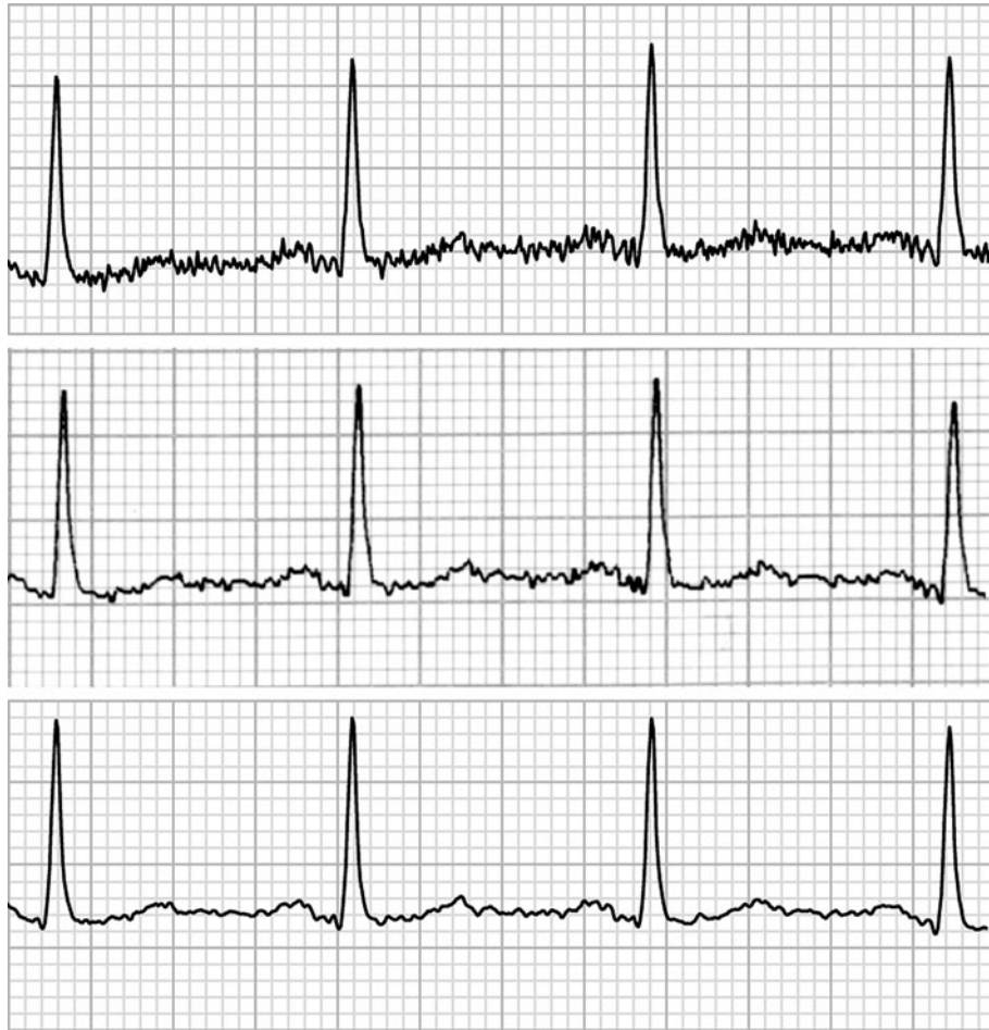
Fig 5. ECG signal processing. The comparisons of ECG signal processing between Philips paper-based ECG and SWT-processed ECG are shown. An original noise-interfered ECG signal is shown in the top panel . The Philips processed ECG is shown in the middle panel . The SWT-processed ECG is shown in the bottom panel . Both Philips processed ECG and the SWT-processed ECG can keep the characteristics of the original ECG in amplitude, duration, and shape.
