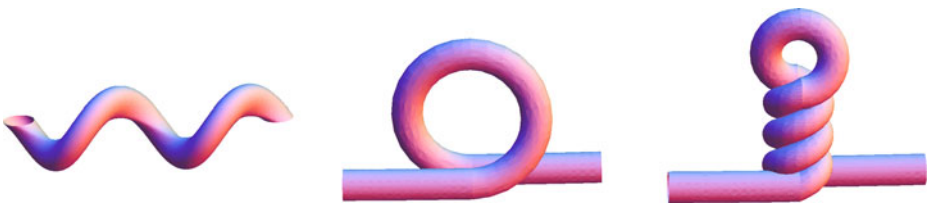
Fig. 1 Cascade of deformation transitions upon increase of the applied twist, from left to right: thin helix, one-helix-turn loop, and rotated loop state
