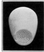
Fig. 7 Gooch crucible showing perforations in the bottom.
