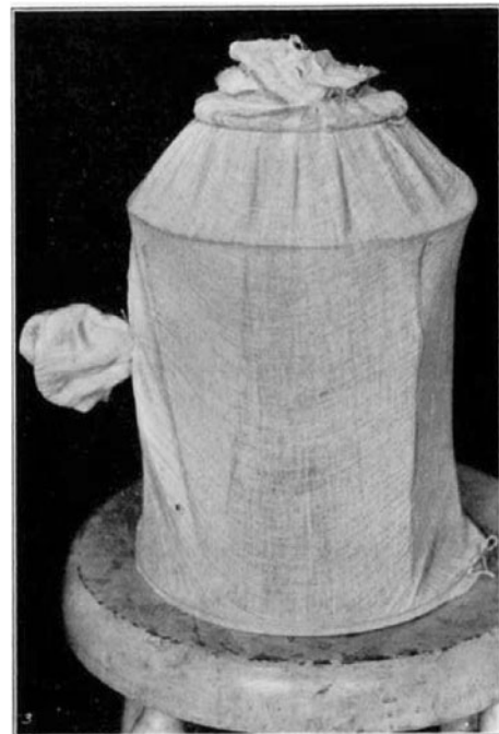
Fig. 9 Cage for housing the flies. The side sleeve is used when feeding or catching the flies. When transferring the flies from one cage to another the top opening is untied and a clean cage is inverted over the old one. A light is placed over the top cage and the flies will at once fly into the clean cage. When they have all been captured the gauze can be drawn together and tied.
