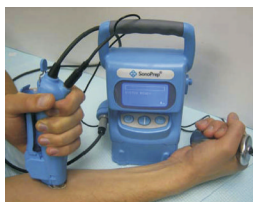
Figure 4. Low-frequency ultrasound treatment in a clinical setting with the SonoPrep® device (Echo Therapeutics, Franklin, MA). The patient holds a conductive polymer hand-piece and the device automatically stops when the skin impedance is decreased to the desired treatment level. Usual treatment times are on the order of 10 seconds (reprinted with permission from Ref. 87).
