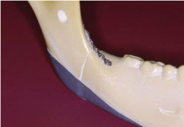
Figure 1 The polyurethane synthetic mandible replica reconstructed with a five-hole microplate and monocortical self-tapping, 1-mm outer thread diameter screws. Note the simulated pterygomandibular sling (using duct tape), intended to mimic minimal soft tissue stripping.
