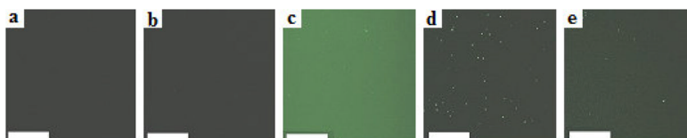
Figure 4. Fluorescence microscopy images after incubating thermally immobilized PEG 20,000 (a); PEOX 200,000 (b); PS 280,000 (c); piranha-cleaned silicon wafer (d); and PFPA-functionalized wafer (e) in BSA-FTIC. Scale bars: 100 \mu\text{m} .
