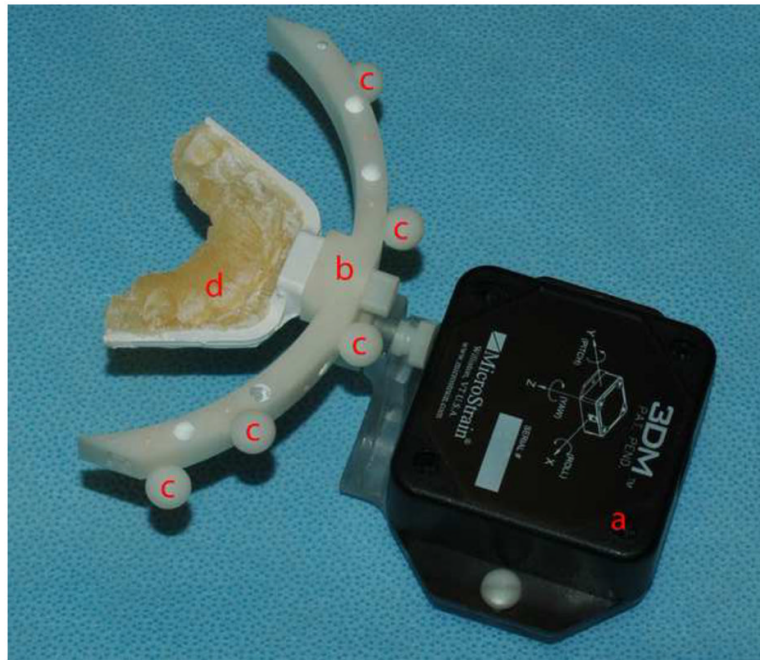
Figure 2. NHP recording device assembly a. The digital orientation sensor b. The facebow c. The built-in fiducial markers d. The individualized bite jig
