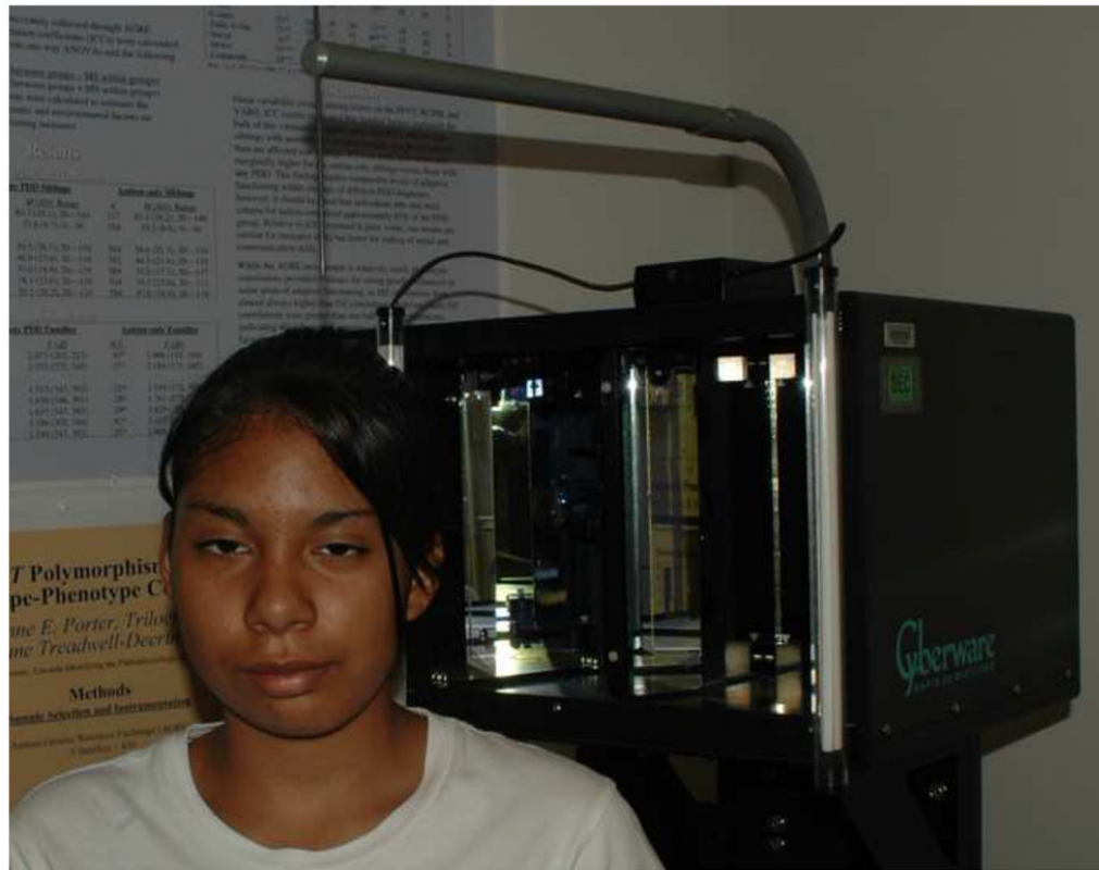
Figure 4. The 1 st NHP is recorded using the laser scanning method when the digital orientation sensor, the bite jig and the facebow are not attached to the patient.
