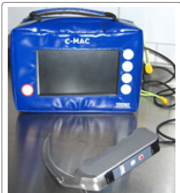
Figure 1 The portable C-MAC videolaryngoscope. The C-MAC videolaryngoscope, stored in the portable protective bag. Note the buttons for image recording on the monitor and the laryngoscope handle.
