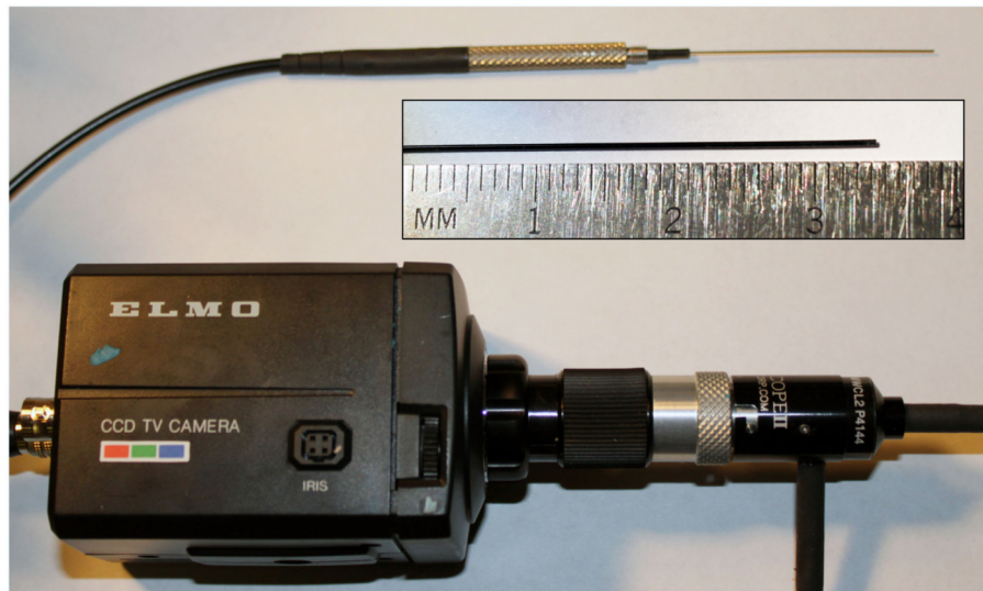
Figure 1. Flexible fiberoptic microendoscope (Zibracorp, Westport, MA): 0.3 mm outer diameter, visualization channel only, 0.4 mm outer diameter including light channel). Length: 62 mm, focal length: 1 mm, 50° FOV, ~50 × magnification; shown attached to color CCD TV Camera (ELMO, Plainview, NY, USA). The small inlet shows the tip of the endoscope next to a millimeter scale.
