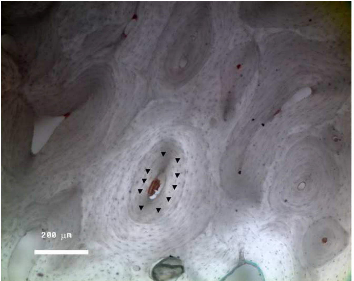
Figure 1. Typical surface of the osteonal cortical bone following polishing. The locations of the indents are marked by a triangle ( \blacktriangledown ), which were midway between the Haversian canal and the edge of the osteon.
