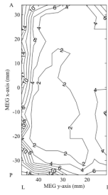
Fig. 7. Contour map showing reconstruction error (mm) of right source as a function of position of left source within suppression region.
