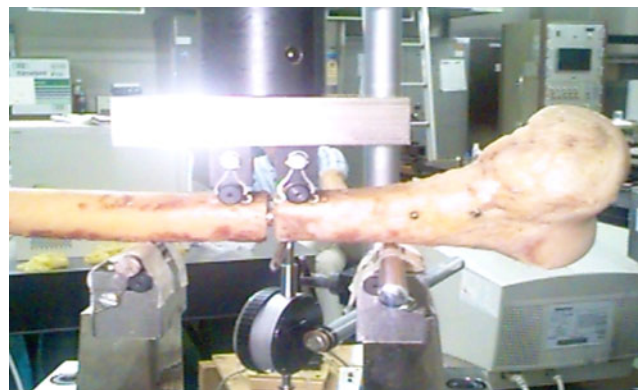
Fig. 2 Four-point bending test performed until the fracture bent to 5-mm displacement
