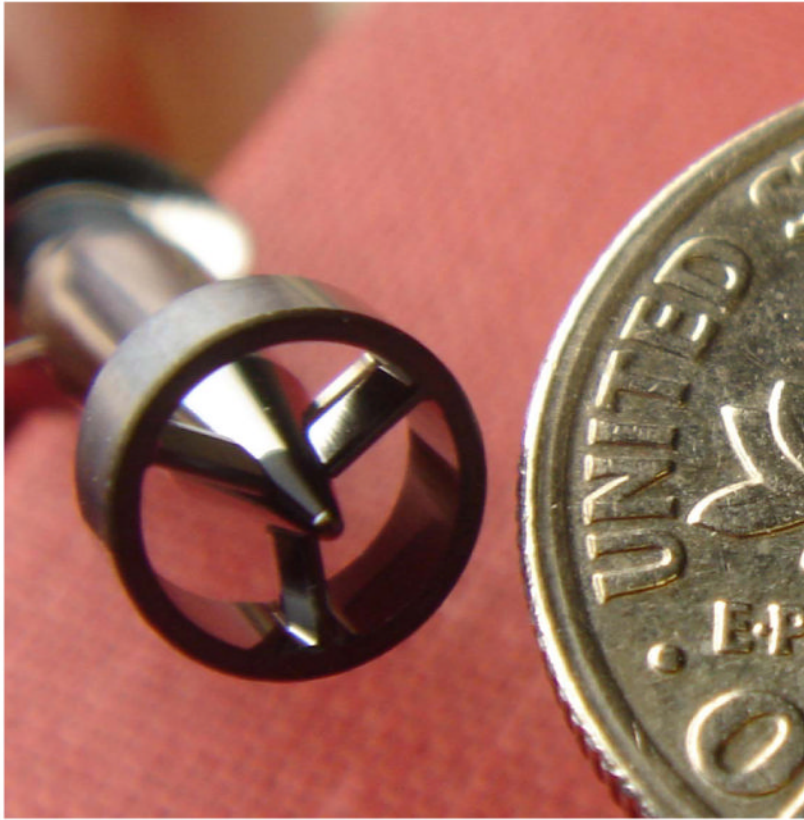
Figure 4. The cone bearing developed for the Infant and Child Jarvik 2000 VADs. The novel design eliminated thrombosis in the bearing during chronic animal studies.
