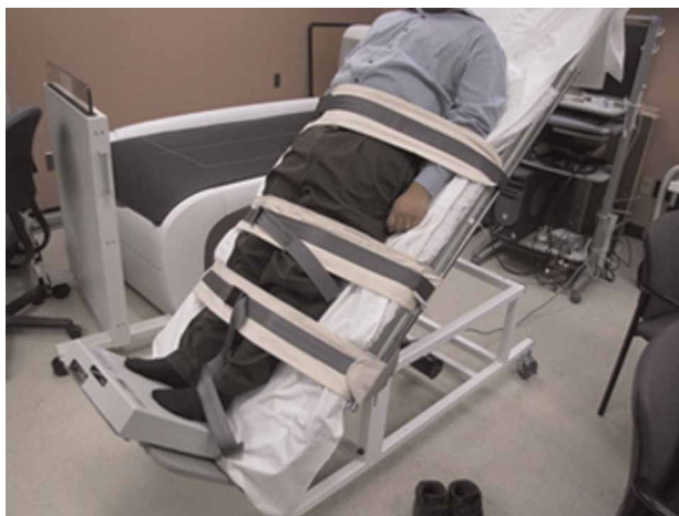
Figure 1 The setup of a supine study subject tilted to 45° and loaded onto a vibration plate. The vibrating plate is located on the foot rest of the tilt table. The straps to secure the subject have been placed in three locations: below the patella, above the patella, and across the trunk.
