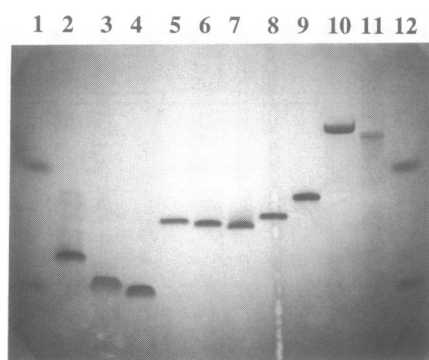
Figure 6. Polyacrylamide gel of disulfide-bridged duplexes and hairpins. Lanes 1 and 12, bromophenol blue and xylene cyanol markers; lane 2, unmodified 12mer control; lane 3, unmodified self-complementary sequence 10 ; lane 4, bridged hairpin 4 ; lanes 5-7, bridged duplexes 3 , 6 and 7 respectively; lane 8, bridged sequence with large loop ( 8 ); lane 9, unmodified 24mer control ( 13 ); lane 10, putative dimer from the oxidation of 9 ; lane 11, unmodified 48mer control.
