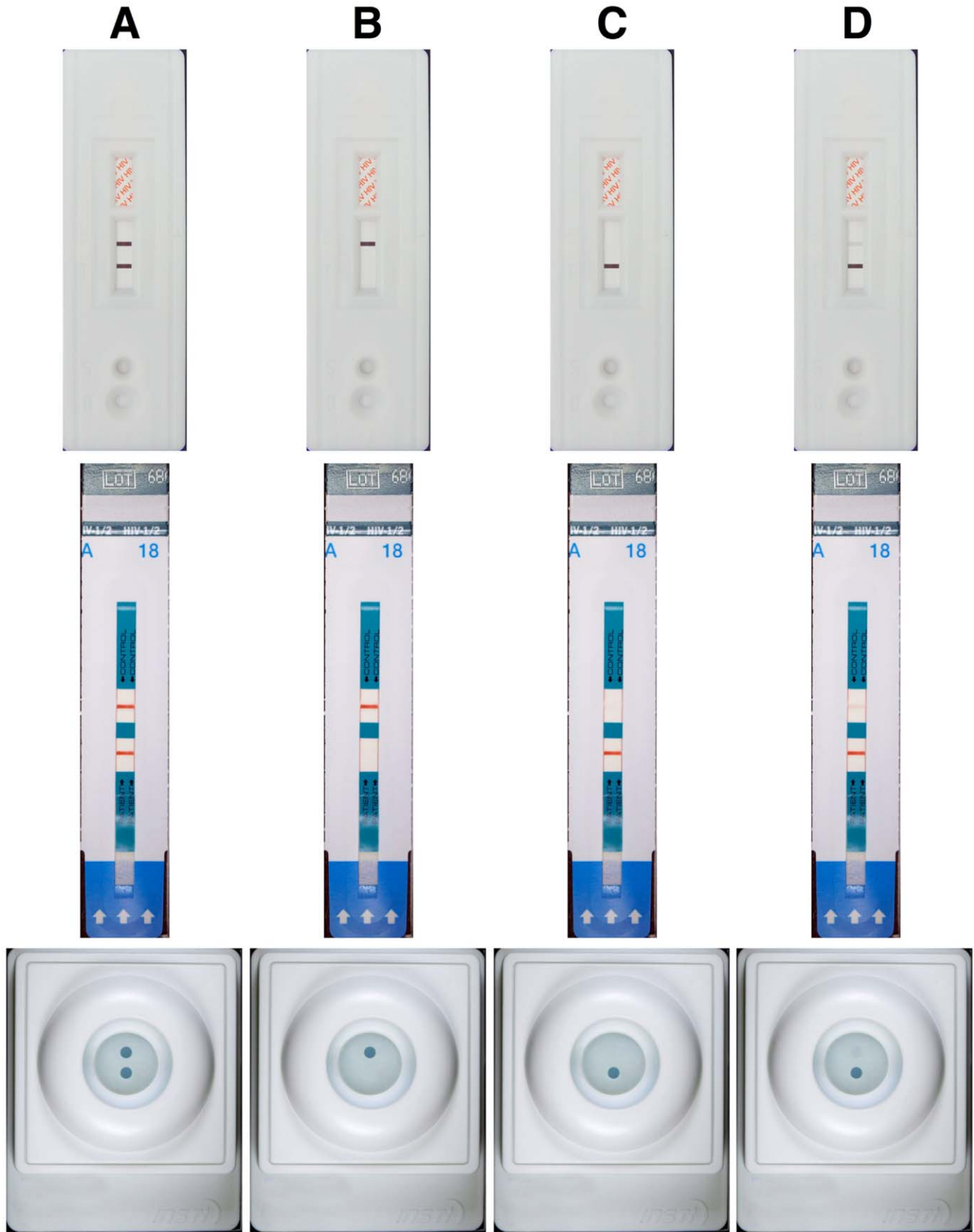
Figure 3. Possible types of result for two-line/dot HIV rapid diagnostic tests (RDTs). RDTs from top to bottom are: Advance Quality, Determine and Insti. Typical results for reactive (A), non-reactive (B) and invalid sample results (C) as shown in manufacturers' instruction were considered "obvious". The results labeled D were considered "difficult" because of the presence of only a faint line/dot and because both lines/dots are not the same intensity. doi:10.1371/journal.pone.0018294.g003
