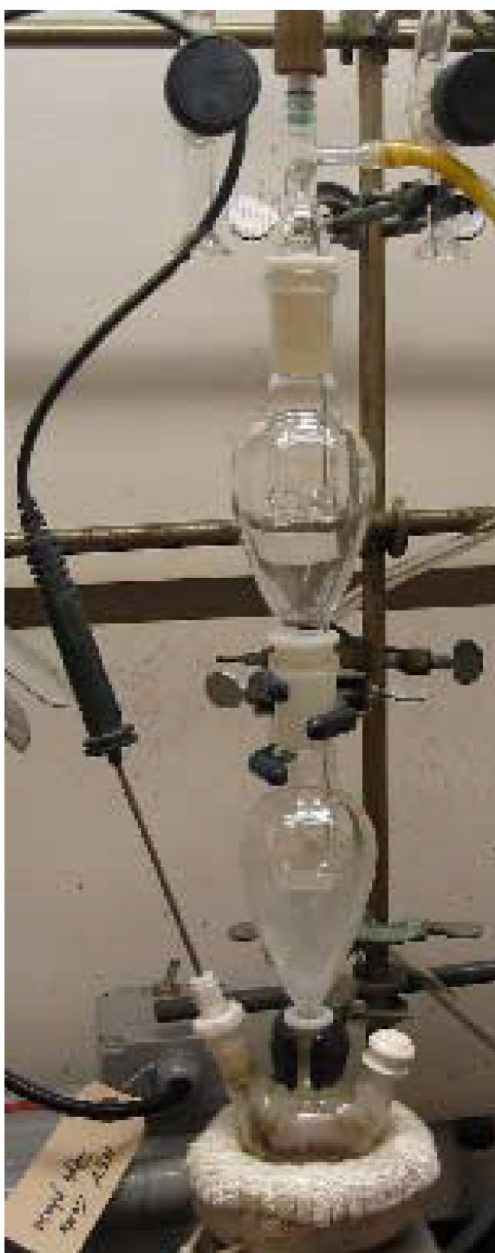
Figure 2. Typical experimental set up for the synthesis of nanocrystals
