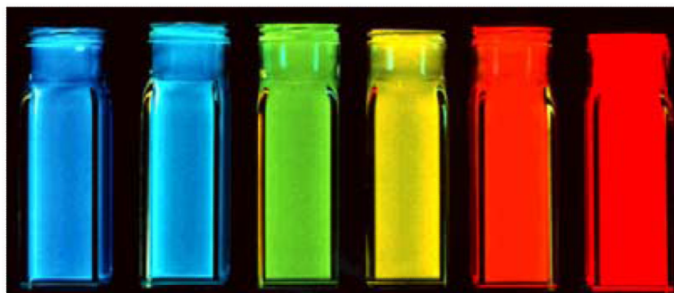
Figure 4. Series of highly fluorescent CdSe/ZnS core/shell nanocrystals (Bawendi) The emission can be tuned from blue through red depending upon the size of the core CdSe nanocrystal.
