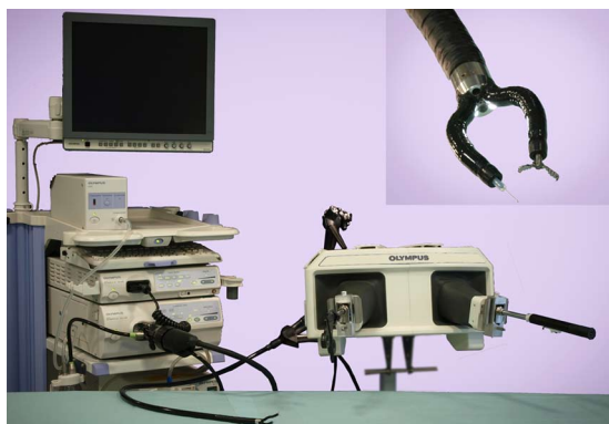
Figure 4 EndoSamarai is a prototype, advanced platform in development by Olympus. To operate the system, a surgeon uses an intuitive, bi-manual interface to control instruments with multiple degrees of freedom (inset shows close-up of endoscope tip with working instruments). Image used with permission (©Olympus Medical Systems Corp.).
