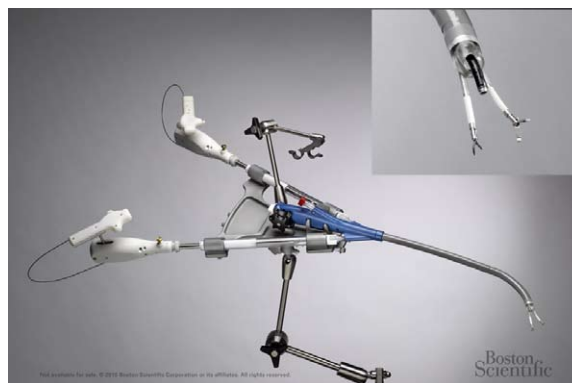
Figure 5 Direct-Drive Endoscopic System from Boston Scientific is a prototype, advanced multi-channel platform currently in development, featuring instruments with multiple degrees of freedom controlled through a bi-manual user interface. Inset figure shows close-up of device tip with a small diameter flexible endoscope in place. Image used with permission (©Boston Scientific).
