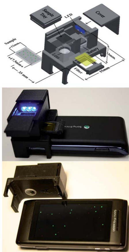
Fig. 1. (Top) Schematic diagram of the designed optical attachment for wide-field fluorescent imaging on a cell-phone. (Middle and Bottom) Different views of the fluorescent imager prototype. This entire attachment to the cell-phone weighs \sim 28 g ( \sim 1 ounce) and has dimensions of \sim 3.5 \times 5.5 \times 2.4 cm. This compact and light-weight unit can be repeatedly attached and detached to the cell-phone body without the need for any fine alignment, making its interface fairly easy to use.
