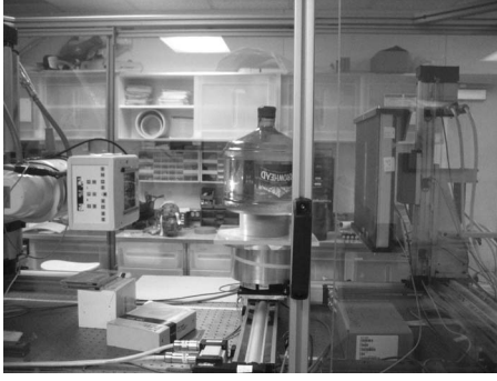
FIG. 4. The tabletop cone-beam CT system with a 260 mm diameter water phantom.
