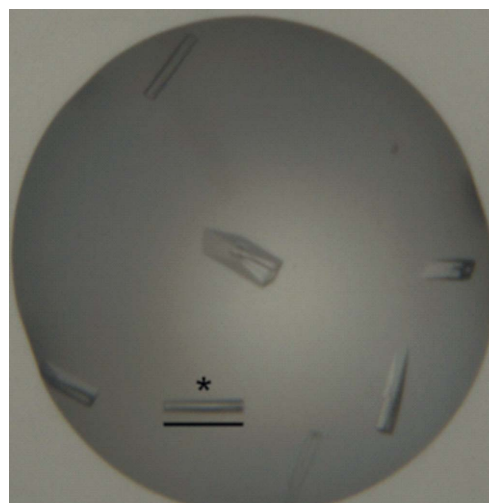
Figure 3 Crystals of DapL grown in JCSG+ condition H9. The scale bar indicates 0.2 mm.
