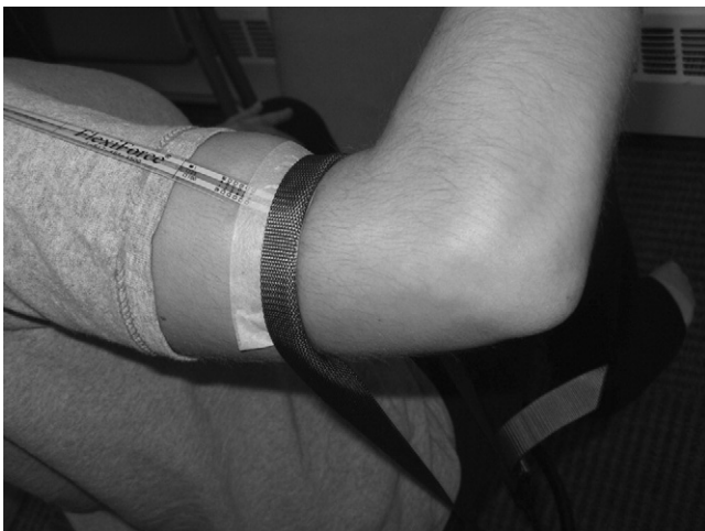
Fig 2. Sensor and strap for measurement of MVIC.
