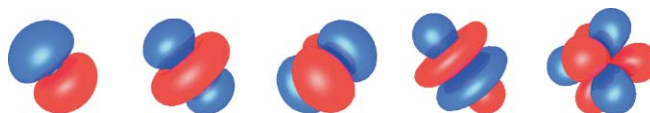
FIG. 1. Charge distributions of moments, from left to right: \mu_0 , a linear dipole; \Theta_0 , a linear quadrupole; \Theta_2 , a square quadrupole; \Omega_0 , a linear octupole; and \Omega_2 , a cubic octupole, in which positive charge is blue and negative charge is red.
