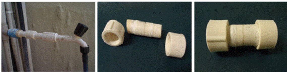
Figure 5. From left to right: (1) sampler device in place, (2) units of samplers to be connected to each other and (3) closed devices for transportation after a suitable period of time.
