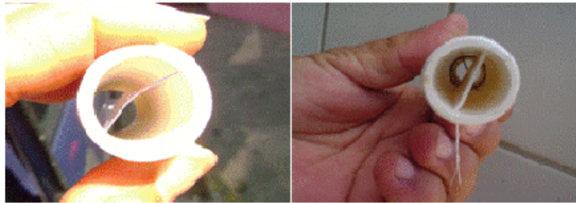
Figure 4. Sampler devices consisted of a hollow PVC pipe within acetate (left) or polyethylene (right) coupons.
