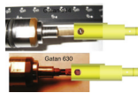
Fig. 1. Gatan 914 cryo-sample holder uses 3 mm diameter round grids, and Gatan 630 holder uses rectangular grids with a width of 3 mm. The anti-contaminator coaxially fits both holders. There are two holes on its side wall, which allow the X-ray beam to illuminate the sample grid and the diffraction signal to propagate without being obstructed.
