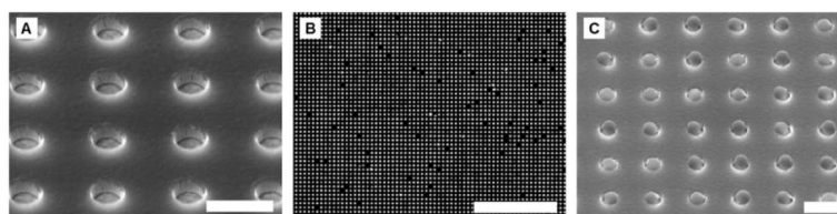
Fig. 4. Arrays of microwells and antibody-conjugated microbeads. (A) SEM image of a small portion of an array of \sim 0.5 \mu\text{m} wells at a 1.2 \mu\text{m} pitch etched in a silicon dioxide film that was deposited on a gold-coated wafer. (B) Raw fluorescence image of a small portion of an assembled array of 0.4 \mu\text{m} antibody-conjugated beads at a 1.2 \mu\text{m} pitch. (C) SEM image of a small portion of an assembled array of 0.4 \mu\text{m} antibody-conjugated beads at a 1.2 \mu\text{m} pitch. The scale bars in (A) and (C) are 1 \mu\text{m} . The scale bar in (B) is 24 \mu\text{m} .
