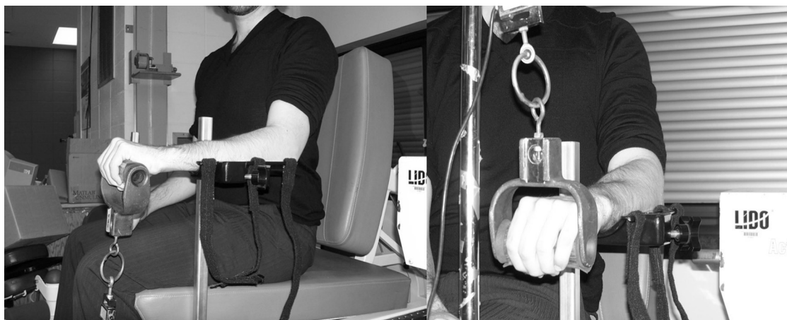
Figure 2 Maximal isometric contraction during wrist extension (left picture) and wrist flexion (right picture).
